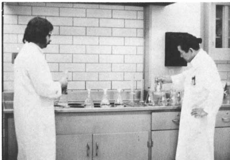
Figure 10. Chemists making threshold odor tests
